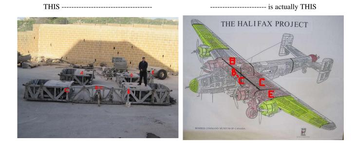
Remember that everything above (in light red) on the Halifax cutaway is what we have acquired and that which is (yellow) has been located. "B" is the right wing box and main spar, "C" is the left wing box and main spar, "E" is the intermediate wing section, and "B-C" is the middle main spar section. "A" and "D" are extra center section wings boxes we recovered. (We have the Boulton-Paul tail turret recovered from the UK and on display at the Bomber Command Museum of Canada in Nanton)
