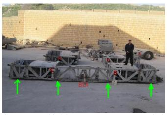
Halifax-Hastings wings recovered in Malta – note green arrows pointing out the main spar.
