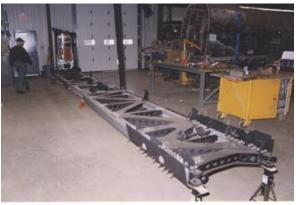
Main Spar table jig for NA337 rebuild
