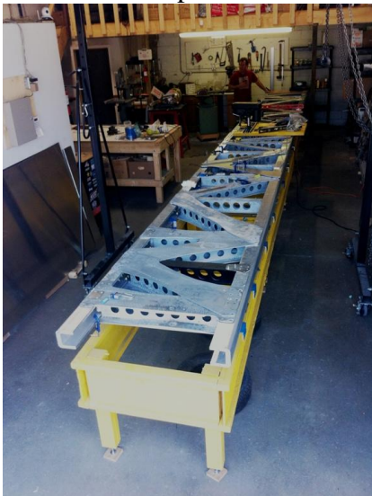
The 30 foot Main Spar almost rebuilt
